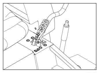
Place controls in neutral position and engage the parking brake.
